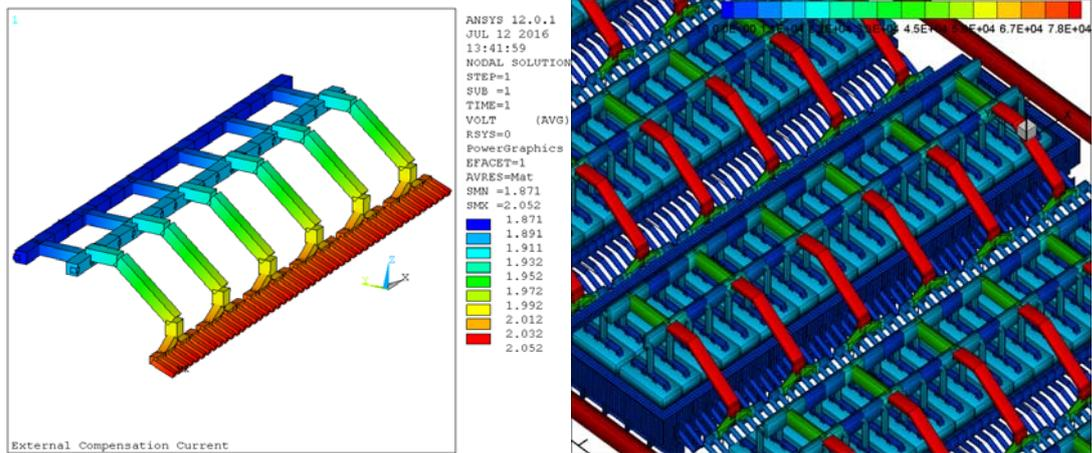
**Figure 9. ECC busbar network concept with 100 % downstream side current exit.**
