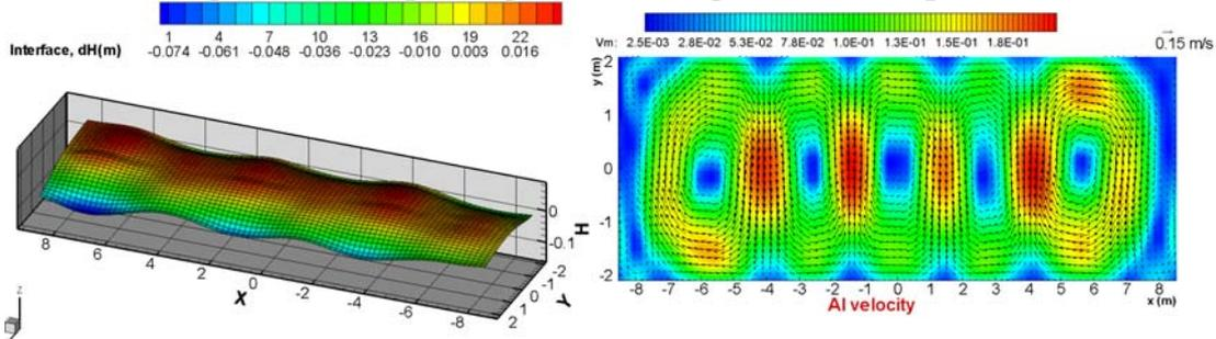
Figure 8. Corresponding steady-state bath-metal interface deformation and steady-state metal pad flow velocity field.
